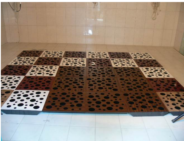
Picture 5: test samples in the reverberation room.
